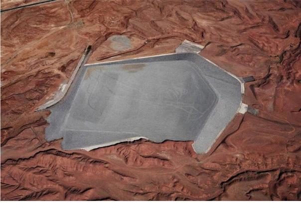
**Uranium Disposal Cell containing 1.3 million tons of toxic waste and uranium tailings, along with the mill, buildings, and a schoolhouse, constructed from contaminated material, Mexican Hat, Utah**
